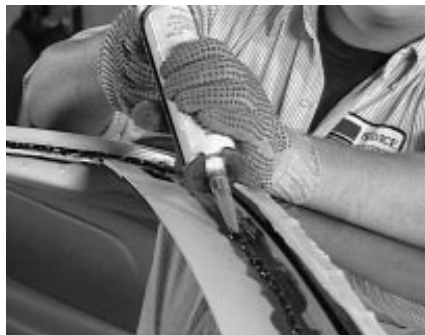
Figure 2—Vehicle makers now recommend adhesive joints on only a few parts, such as some metal roof panels. (Courtesy of GM)
