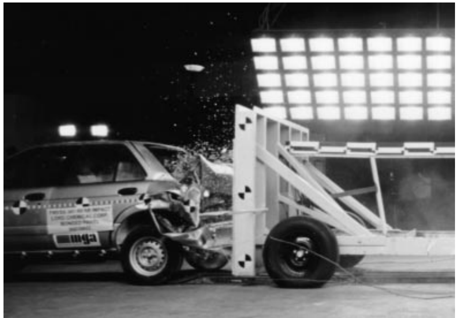
Adhesively bonded panels were compared to welded panels in FMVSS 301 crash test. (Courtesy of Lord Fusor)
